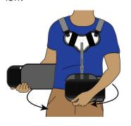
3. Grasp both right and left pull handles and pull them simultaneously to tighten them, then lay them down on the front of the brace.
